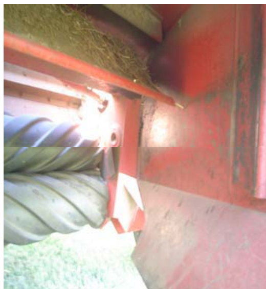
Figure 6: Correct spacing and tension on the conditioning rollers (left), and adjustment of the crop deflector (above) and windrow forming shields (right) result in quick drying with minimal crop damage.
